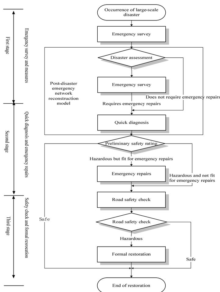
Figure 1. The emergency network reconstruction process (Lin *et al.*, 2002)
